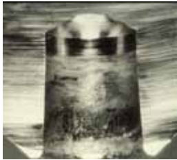
Surface damage to a head/neck taper
