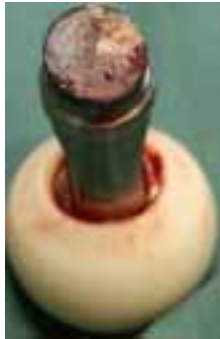
Surface damage to a head/neck taper
