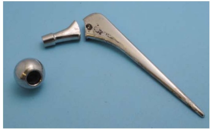
Fig 2: The prosthetic stem fracture propagated inferiorly from its origin at the insertion "dimple".
