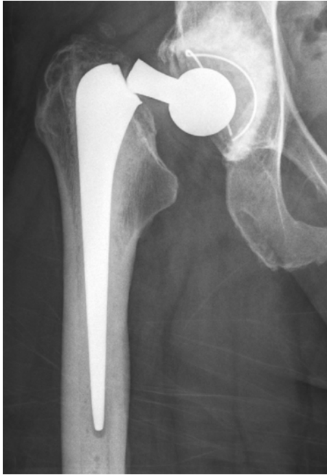
Fig 1: Prosthetic fracture of a polished, tapered, collarless femoral stem; a cemented polyethylene cup has been used.
