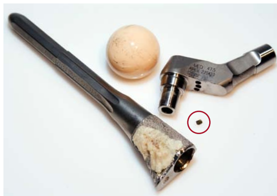
Figure 8. Retrieved Apex Modular Stem showing broken locating pin with no other apparent damage to Dual Press Modular Junction. Note: Good bone attachment to porous surface. (Courtesy JISRF Archives)
