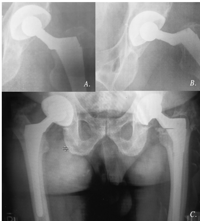
Figures 7A, B, and C. A: Post-op A/P X-ray of a fractured locating/de-rotational pin. Note: is difficult to appreciate the pin has been broken on this view. B: Lateral X-Ray demonstrating modular shoulder/neck component has rotated out of position of function. C: A/P x-ray showing bi-lateral hips with Apex Modular stem on the left side, and a S-Rom (primary stem-length) that replaced the fractured locating/de-rotational pin on the right. (Courtesy T. Tkach)
